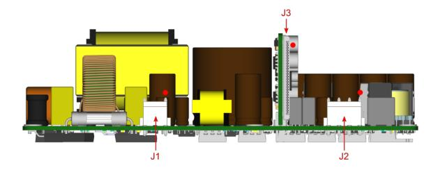
Please note above drawing is made from an early prototype exact locations and connector pinout is not representable for the current hardware. J3 is moved to the daughter board and is now a 26-pole 1mm pitch FPC connector.
