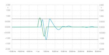
Green line: GlidePath 200Hz 1 cycle. Blue line: actual cone excursion. At the first part of the sine, the cone goes up to 0,7V and drops down to -1,13V in the second part and goes up again to 0,74V as the signal stops.
