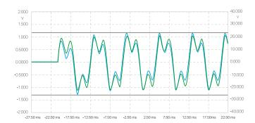
Competitor driven with 5 cycles of 60Hz mixed with a 180Hz/-6db signal. The graph shows that the output initially has less voltage at the first part of the sinewave, but overshoots on the negative side. This effect fades out gradually in the next cycles. The loudspeaker receives peak levels of +22,85V and -25,1V. The deviation between plus and minus peak levels is about 10%.
