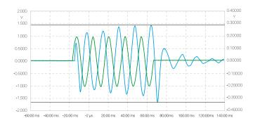
DirectDrive module driven with a 50Hz 5 cycles burst. The GlidePath direct drive architecture has a peak cone excursion of +286mv and-308mV. The trail output after the signal stops has a peak output of 80mV
