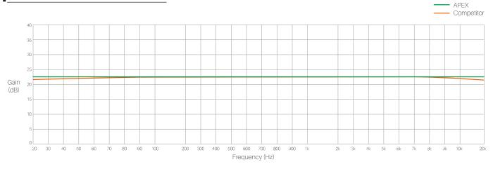
In the comparison frequency response, we can see that both responses are nearly flat apart from a slight roll-off at the high and low extremes. This is more than sufficient flat to power a speaker with an intended response from 60Hz-16K. The Apex GlidePath architecture has a -3dB point of 2Hz, the competitor has a -3dB point of 15Hz.
