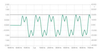
Apex GlidePath driven with 5 cycles of 60Hz mixed with a 180Hz/-6db signal. The graph shows barely any deviation between input and output. The loudspeaker receives peak levels of +20,4V and -21,9V. The deviation between plus and minus peak levels is about 5%.
